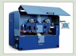
with splinter guards and anti-kickback devices. **Press**: the rollers that make up the press are operated by pneumatic cylinders with adjustable pressure. 10,4 inches touchscreen control panel.
