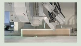
**zero overspray**, a flat and accurate application blade, and minimum footprint. The solution is ideal to paint edges of any shape and size, including non-throughpass door handles that would be impossible to paint using other systems.
